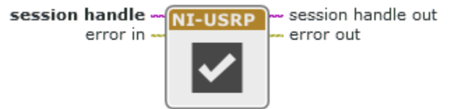
Figure 16: "niUSRP Commit" block for validation of properties to the USRP device.
