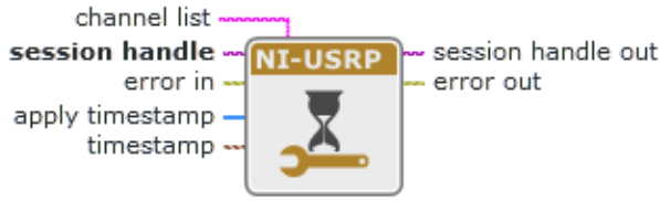
Figure 19: “niUSRP Set Time” block forgetting the time with the onboard timer.
